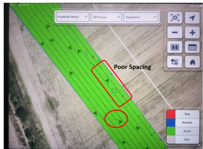
Figure 2. Planter singulation of each treatment, as monitored by the Climate FieldView™ Cab app.
