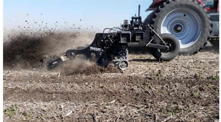
Figure 3. A strip-freshener runs at speeds of five to 10 miles an hour and conditions the top two inches of soil in preparation of planting. Photo used with permission from Yetter Manufacturing.
