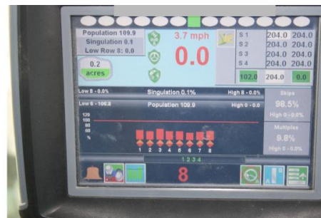
Figure 2. Using predetermined data from a "Skipulator," planters were programmed to randomly insert skips into each planting population.
